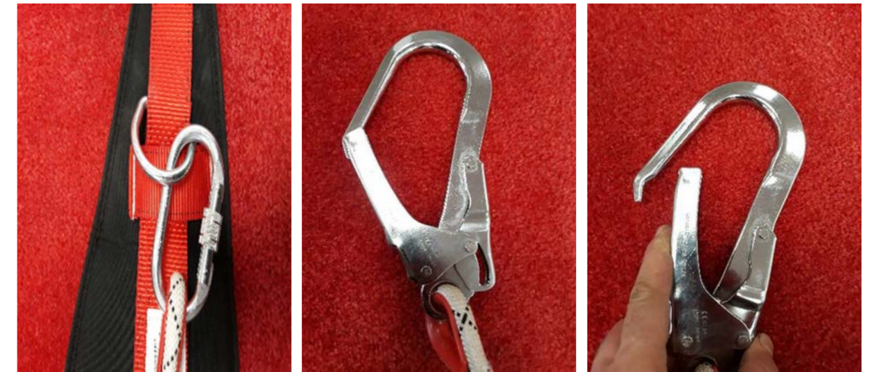
The lanyard is secured to the belt by means of a screw gate karabiner. Ensure that this is tightened securely.
